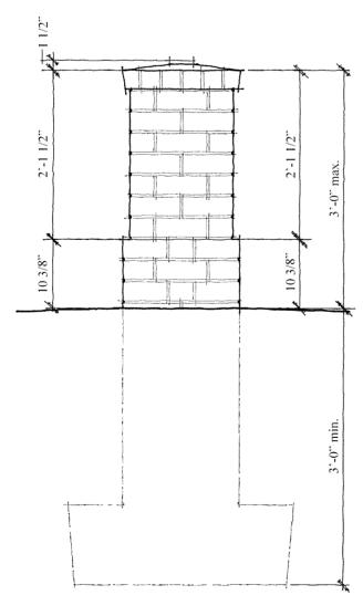
Standard Brick Pier Elevation Scale: 3/4" = 1'-0"
